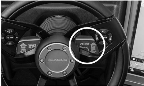
This switch allows the speed of the boat to be increased or decreased while the Zero-Off is engaged.
