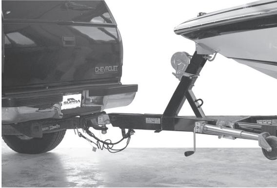
**NOTICE: If your hitch ball has an excessive flat spot on top, the latch may not engage properly. If the latch does not catch, check with your dealer or hitch installer before trailering.**
