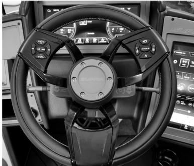
The remotes must be paired with the ICE Audio control. See the Vision Touch manual if the controls are not working.
