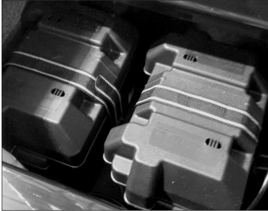
The battery is mounted under the port side cushions. Location may vary slightly depending on the model.
