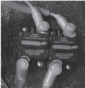
To turn off the power to the PDM's, manually press the red button and the circuit breaker reset lever will flip open and the power to the PDM's will be shut off. To reset the circuit breaker, push the reset lever closed.
