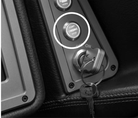
Located on the right side of the dashboard, the ignition switch has four positions. In the vertical position the ignition is “OFF”. In the OFF position, only the blower and bilge pump switches are powered.
