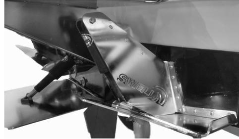
The Swell System utilizes actuator operated plates to create wake shape. The Plates are controlled by the VISION system. Please refer to the Supra VISION Touch Manual for more details.
