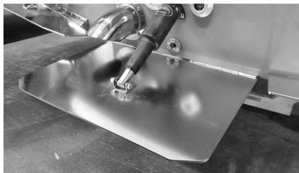
The wake plate allows the driver to control the running attitude of the boat. It can be controlled by the switch on the dashboard.
